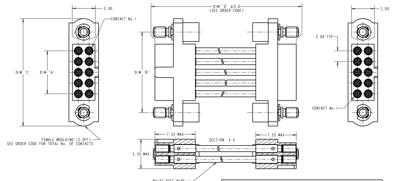
WHITE PTFE WIRE: IN ACCORDANCE WITH COMPONENT SPECIFICATION CO49XX (SEE ORDER CODE FOR WIRE GAUGE)
