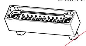
EXAMPLE ORDER CODE: CONNECTOR WITH 20 CONTACTS. GOLD ON CONTACT AREA AND 100% TIN ON TAIL, 2.7mm PC TAIL
