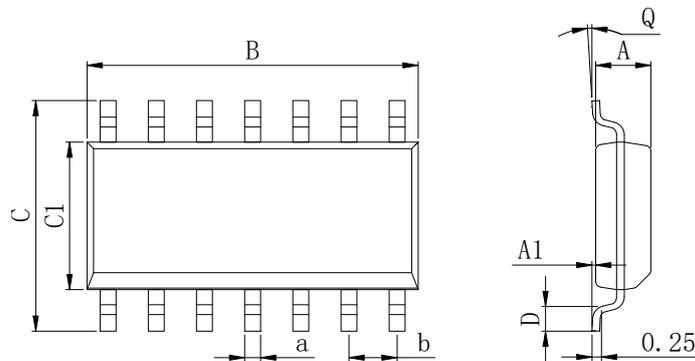
Dimensions In Millimeters(SOP-14)
