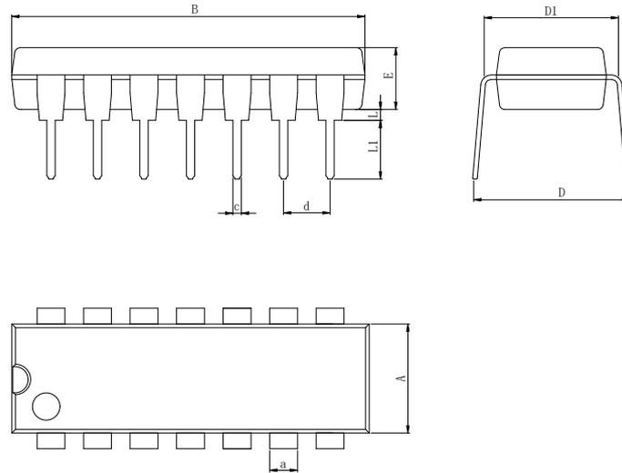
Dimensions In Millimeters(DIP-14)
