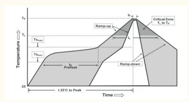
■ Recommended reflow methods: IR, vapor phase oven, hot air oven, N₂ environment for lead-free:
