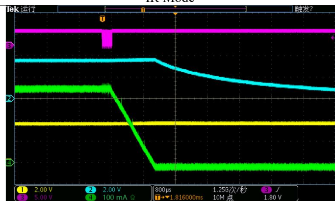
CH1: SW, CH2:VOUT, CH3:VSDA, CH4:ILED Movie Current Ramp Down@ ILED1= ILED2=187mA
