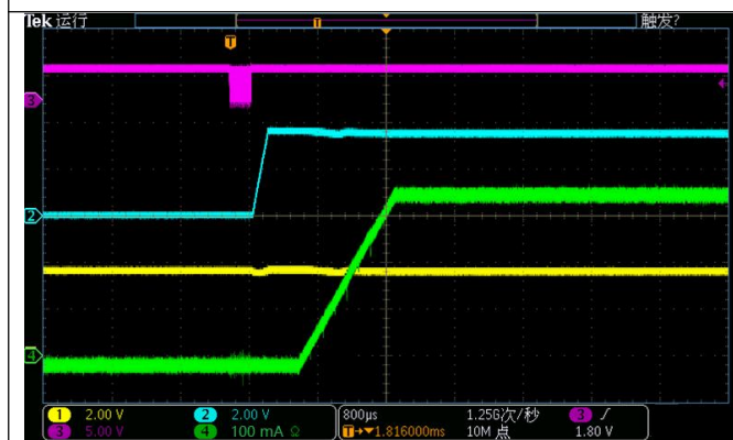
CH1: SW, CH2:VOUT, CH3:VSDA, CH4:ILED Movie Current Ramp Up@ ILED1= ILED2=187mA
