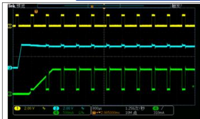
CH1:TX Signal, CH2:VOUT, CH4:ILED TX Interrupt @ ILED1=ILED2=500mA
