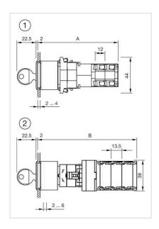
1 = Kraus & Naimer switching element A = (Number of stages x 12) + 66.5 mm 2 = Santon switching element B = (Number of stages x 13.5) + 65.5 mm
