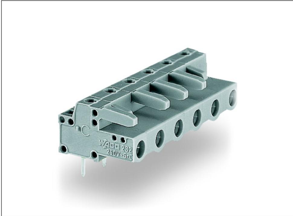
Printview: Female connector; with angled solder pins; 6-pole; Pin spacing 7.5 mm / 0.295 in; Solder pin 0.6x1 mm; codable; Horizontal PCB mounting; with 2 locking latches; with coding finger - Item No.: 232-836
