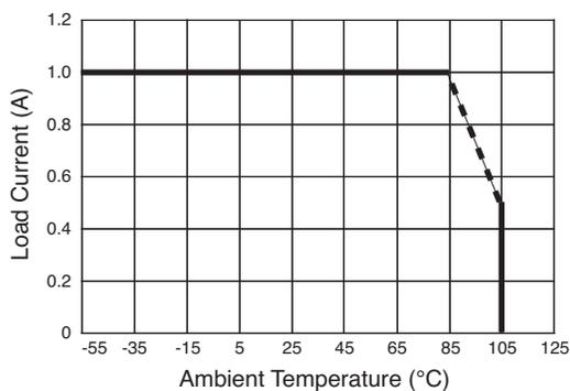
Figure 4 — FR75-1 load current vs. ambient temperature
