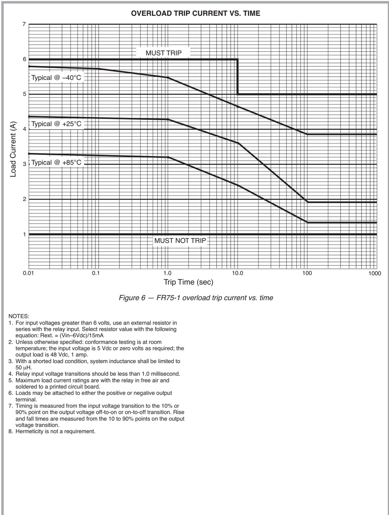
Figure 6 — FR75-1 overload trip current vs. time
