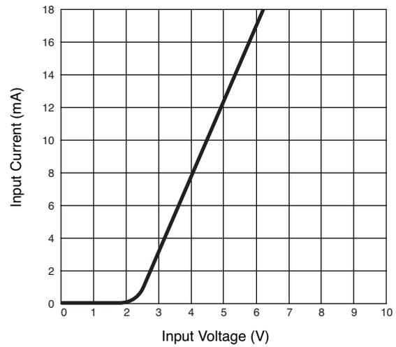
Figure 2 — FR75-1 input current vs. input voltage
