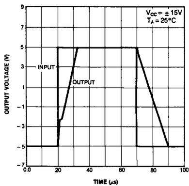
Figure 13. Voltage Follower Large Signal Pulse Response
