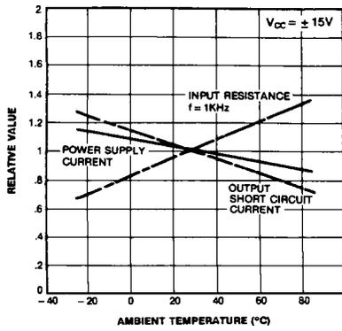
Figure 7. Normalized DC Parameters vs Ambient Temperature
