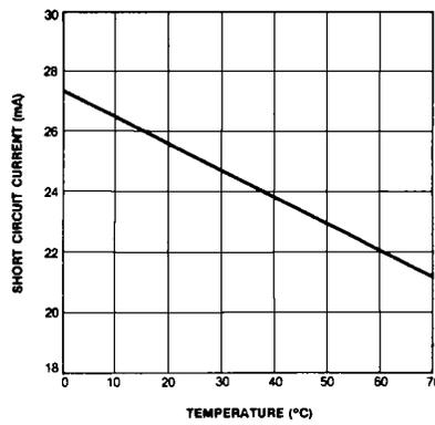
Figure 10. Output Short Circuit Current vs Ambient Temperature
