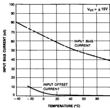
Figure 3. Input Bias Current vs Ambient Temperature
