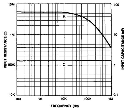
Figure 2. Input Resistance and Input Capacitance vs Frequency
