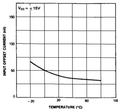
Figure 5. Input Offset Current vs Ambient Temperature
