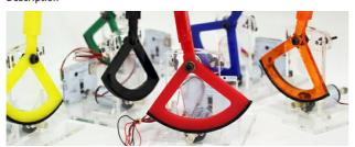
We worked with Stanford University to design the Hapkit Board, which supports the Hapkit open-source haptic device.
