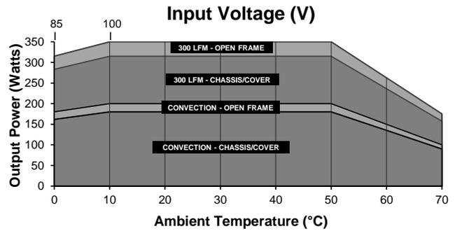
**Derating requirements** – Chart above applies to models 1004 thru 1008 only. 350W 300LFM forced air, open frame. 200W convection cooled open frame. Derate 10% with chassis and cover. Derate 1.5W<sub>OUT</sub>/1V<sub>IN</sub> below 100V<sub>IN</sub> and between 100V<sub>IN</sub> and 85V<sub>IN</sub>. Use larger of the two deratings when using chassis/cover below 100V<sub>IN</sub>. Derate output power linearly to 50% between 50° and 70°C. Refer to model listing for all ratings.
