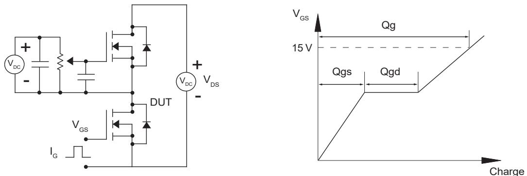
Figure 19. Gate Charge Test Circuits and Waveforms
