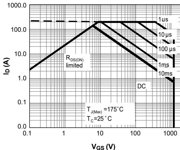
Figure 17. Maximum Forward Biased Safe Operating Area for AOM020V120X2 (Note 1)
