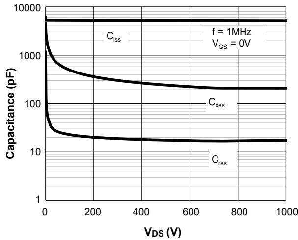
Figure 10. Capacitance Characteristics
