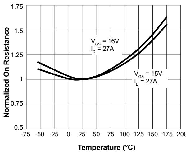
Figure 4. Normalized On Resistance vs. Junction Temperature
