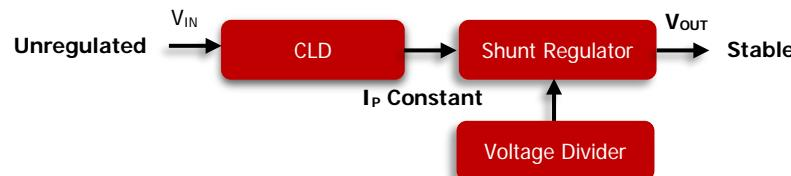
Fig. 4a: Block diagram CLD + Shunt Regulator
