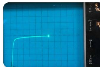
Fig. 3a: I<sub>P</sub> = 24mA at V<sub>IN</sub> = 60V<sub>DC</sub>
