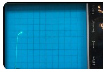
Fig. 2a: I<sub>P</sub> = 28mA at V<sub>IN</sub> = 10V<sub>DC</sub>
