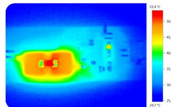
Fig. 2b: T<sub>c</sub> = 53.4 °C at V<sub>IN</sub> = 10V<sub>DC</sub>
