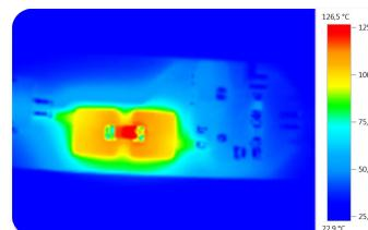
Fig. 3b: T<sub>c</sub> = 126.5 °C at V<sub>IN</sub> = 60V<sub>DC</sub>
