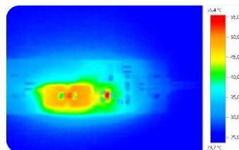
Fig. 5c: Shunt Regulator T<sub>C</sub> = 55.4 °C at V<sub>IN</sub> = 10V<sub>DC</sub>
