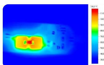
Fig. 5d: Shunt Regulator T<sub>C</sub> = 65.2 °C at V<sub>IN</sub> = 60V<sub>DC</sub>
