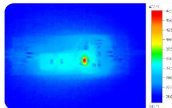
Fig. 5b: Shunt Regulator T<sub>C</sub> = 47.6 °C at V<sub>IN</sub> = 6V<sub>DC</sub>
