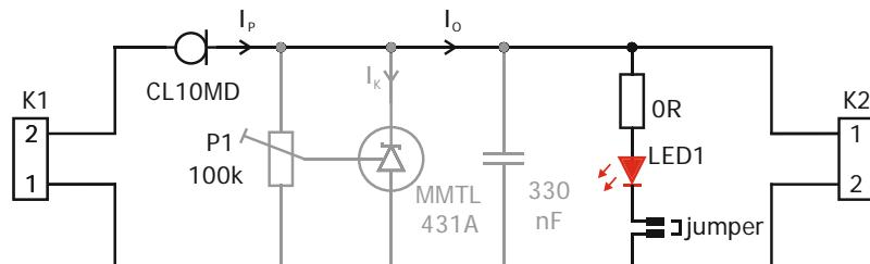
Fig. 1b: Schematic of CLD – LED driver
