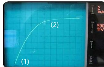
Fig. 5a: CLD. At I<sub>P</sub> = 1mA (start-up), the voltage drop at the CLD is only about 200 mV (1). At 3V drop, already 16 mA are possible (2)
