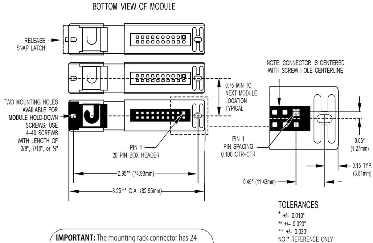
**IMPORTANT:** The mounting rack connector has 24 pins; the module connector has 20 pins. The extra pins on the mounting rack connector prevent misalignment of the module during installation.
