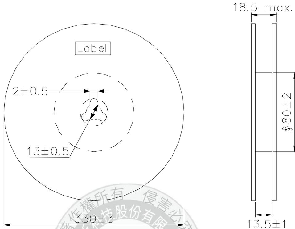
Label position: on the opposite side of sprocket holes side of reel
