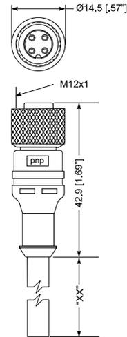
Actuator/sensor cordset, single-ended, M12, 3- and 4poles, female 90° connector with LED operation and function indicator with self-locking thread and molded cable.
