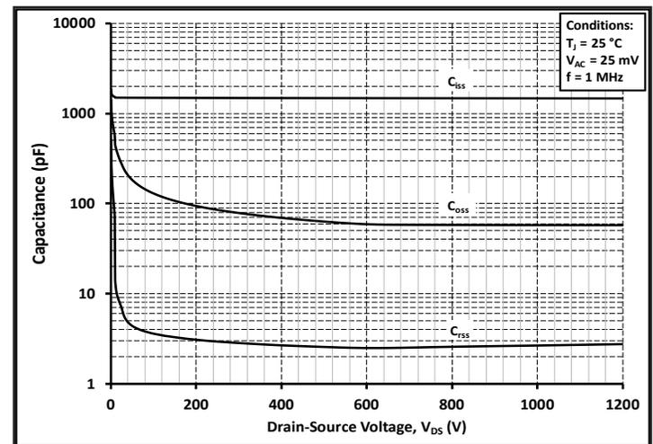
Figure 18. Capacitances vs. Drain-Source Voltage (0 - 1200V)
