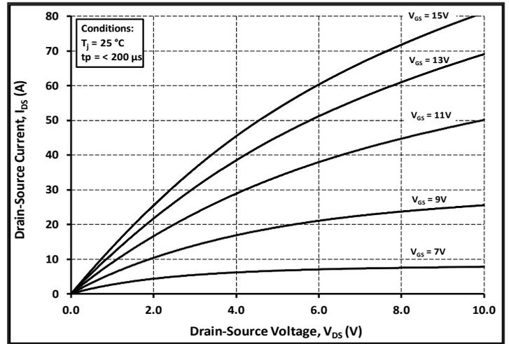
Figure 2. Output Characteristics  $T_j = 25\text{ }^\circ\text{C}$
