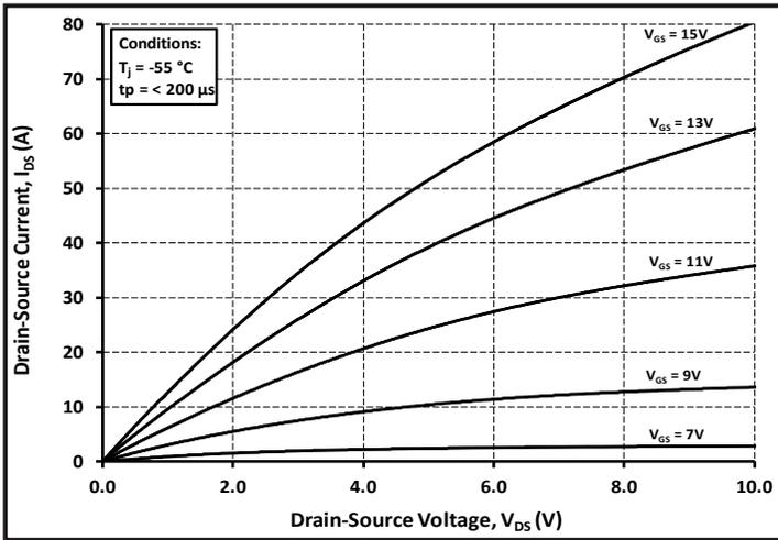
Figure 1. Output Characteristics  $T_j = -55\text{ }^\circ\text{C}$
