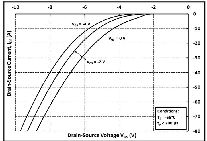
Figure 8. Body Diode Characteristic at -55 °C
