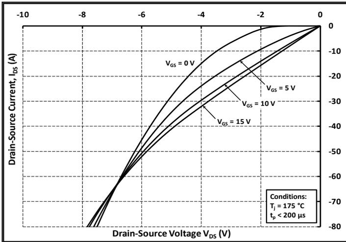
Figure 15. 3rd Quadrant Characteristic at 175 °C
