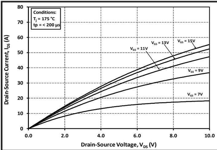
Figure 3. Output Characteristics  $T_j = 175\text{ }^\circ\text{C}$
