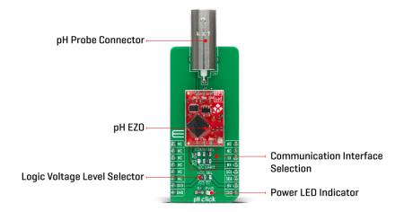
The pH EZO $^{\text{m}}$  circuit is characterized by great sensitivity that gives its accuracy. When electrical noise is interfering with the pH readings, it is common to see rapidly fluctuating readings or readings that are consistently off. To verify that electrical noise is causing inaccurate readings, place the pH probe in a cup of water by itself. The pH readings should stabilize quickly, confirming that electrical noise was the issue.
