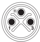
Pin assignment of M12 plug, 3-pos., S-coded, view of pin side
