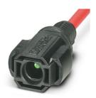
Device connector front mounting, Range of articles: SUNCLIX, housing material: PPE, color: black, number of positions: 1, min. conductor cross section: 2.5 mm<sup>2</sup>, rated voltage: 1000 V DC, rated current: 27 A, Connection method: Crimp, Contact connection type: Pin, cable length: 235
