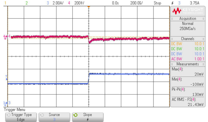
Output Ripple@20MHz BW, Vin = 72Vdc, Full Load with 2200uF output capacitance
