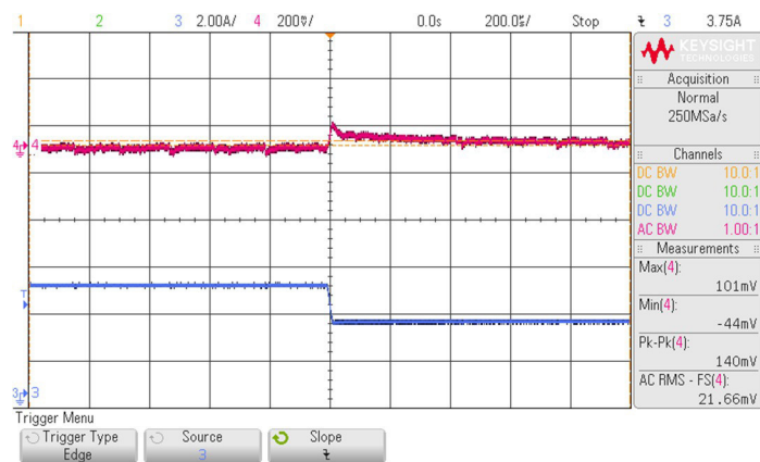
Output voltage response to step-change in load current (50%-75%-50% of full load; di/dt = 0.1A/1s)
