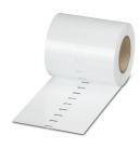
Marker for terminal blocks, can be ordered: by line, white, labeled according to customer specifications, mounting type: snap into universal marker groove, snap into flat marker groove, for terminal block width: 6.2 mm, lettering field size: 6.  $35 \times 6.15 \text{ mm}$
