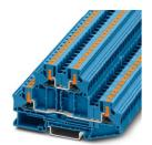
Double-level terminal block, nom. voltage: 1000 V, Thermal continuous current  $I_{th}$ : 28 A, connection method: Push-in connection, 1st and 2nd level, Rated cross section: 4 mm<sup>2</sup>, cross section: 0.2 mm<sup>2</sup> - 6 mm<sup>2</sup>, mounting type: NS 35/7,5, NS 35/15, color: blue
