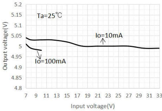
**Output Voltage vs. Load**
