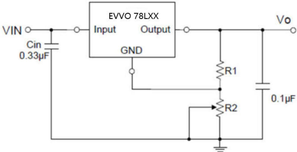
**Fig.3 Adjustable Output Regulator**
