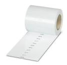
Marker for terminal blocks, Roll, white, unlabeled, can be labeled with: THERMOMARK ROLL 2.0, THERMOMARK ROLL, THERMOMARK ROLL X1, THERMOMARK ROLLMASTER 300/600, THERMOMARK X1.2, THERMOMARK S1.1, perforated, mounting type: snapped, snap into flat marker groove, for terminal block width: 10.2 mm, lettering field size:  $6.35 \times 10.15$  mm, Number of individual labels: 10000
