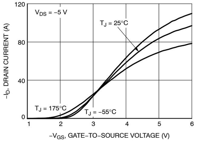
Figure 2. Transfer Characteristics
