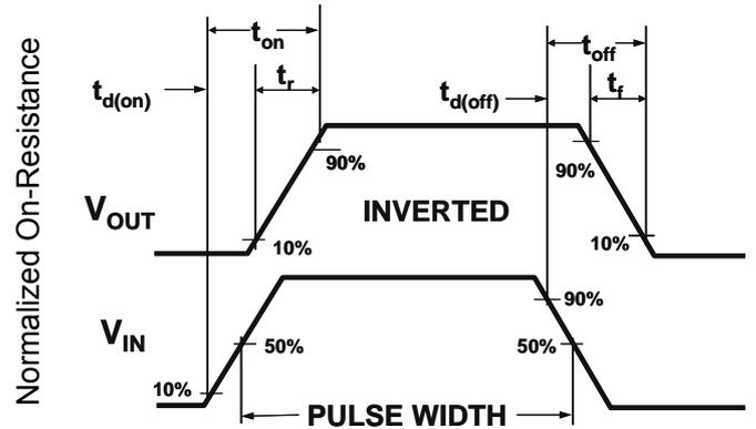
**Figure 2: Switching Waveforms**
