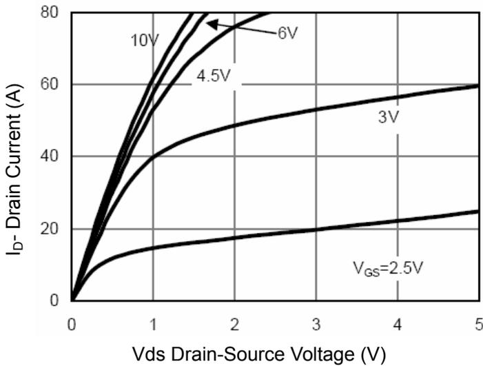
**Figure 3 Output Characteristics**
