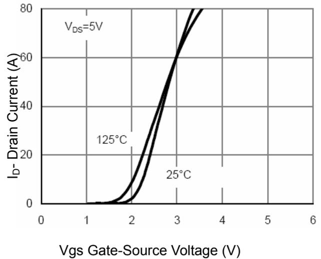
**Figure 4 Transfer Characteristics**
