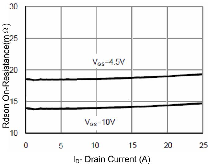
**Figure 5 Drain-Source On-Resistance**
