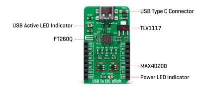
This Click board™ can communicate with MCU via UART or I2C interface. The FT260Q uses the UART interface with commonly used UART RX and TX pins and hardware flow control pins UART CTS and RTS (Clear to Send and Ready to Send) to transmit and exchange data with the host MCU or using the I2C interface, which can also act as a Master with a maximum I2C bus speed of up to 3.4Mbit/s. These two interfaces exist concurrently and can be selected independently according to the application.
