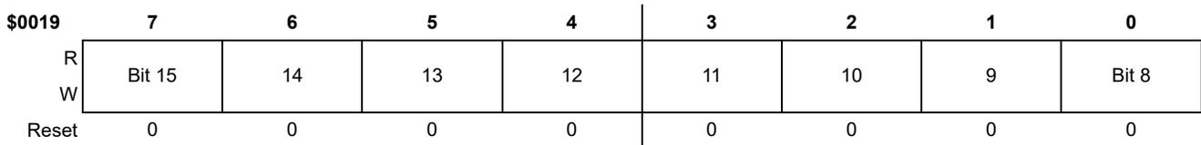
**Figure 52. Timer Channel 1 Value Register High (TPM1C1VH)**
