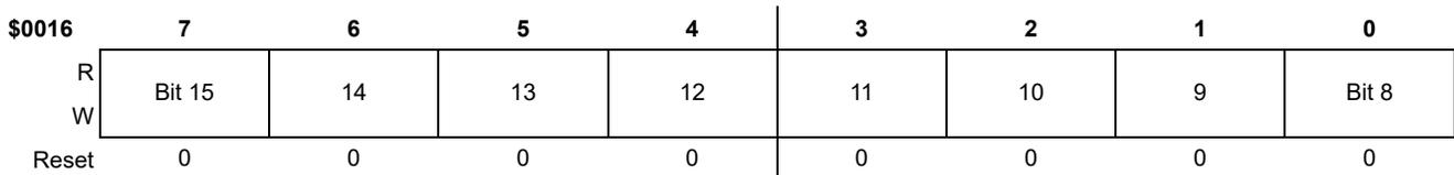
**Figure 49. Timer Channel 0 Value Register High (TPM1C0VH)**
