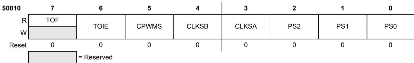
Figure 43. Timer Status and Control Register (TPM1SC)
