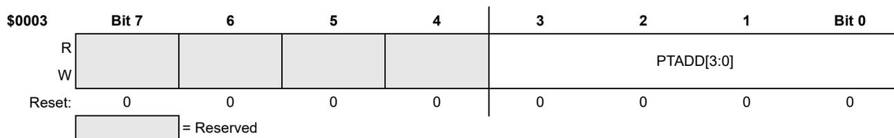
Figure 32. Data Direction for Port A Register (PTADD)
