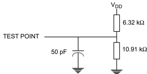
Figure 121. Control Timing Test Load for Digital Pins
