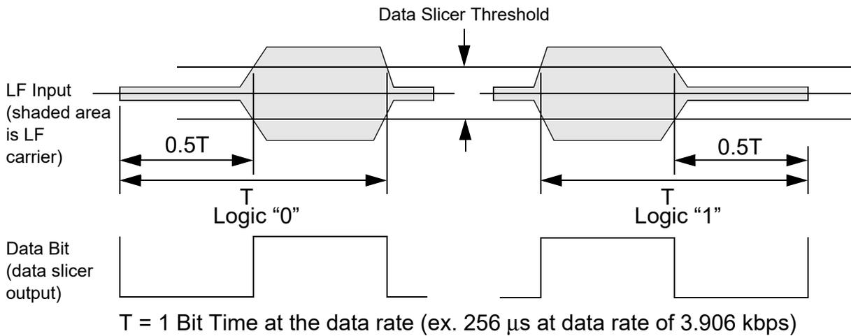
**Figure 68. Manchester Encoded Datagram for LFPOL = 1**
