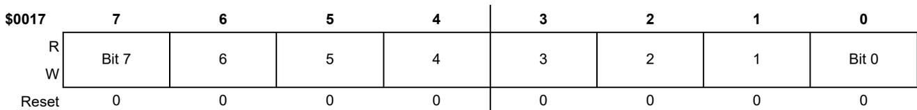
**Figure 50. Timer Channel 0 Value Register Low (TPM1C0VL)**
