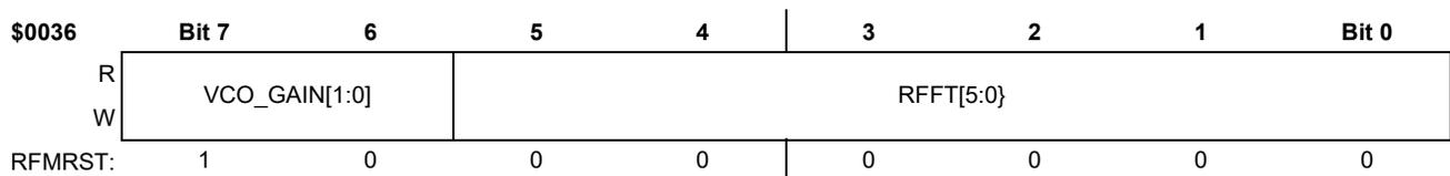
**Figure 105. RFCR6 Register - Frame Number Time - RFTS[1:0] = 1:0**
