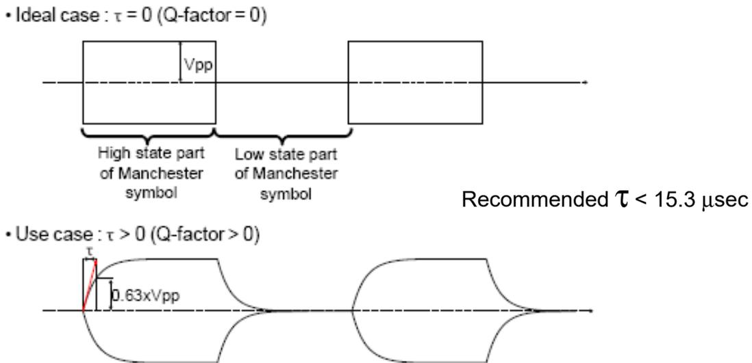
Figure 72. LF Envelope Filtering
