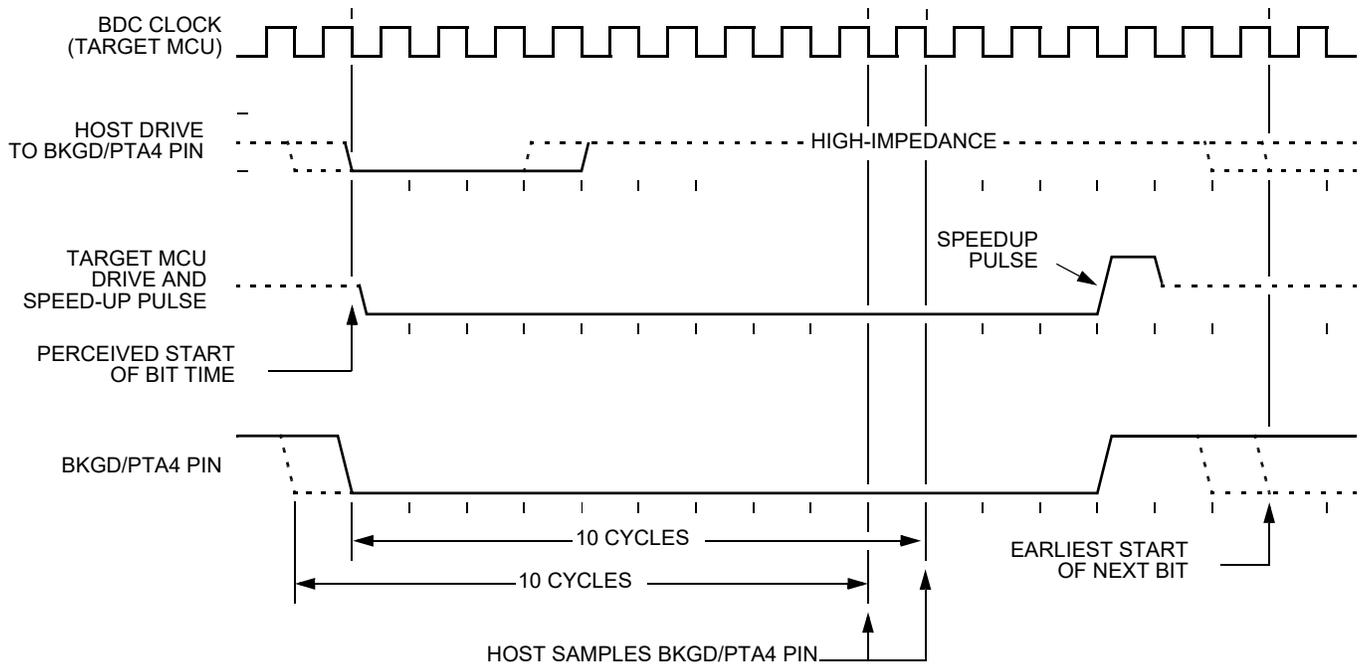
Figure 117. BDM Target-to-Host Serial Bit Timing (Logic 0)
