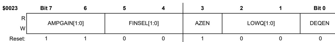
**Figure 86. LFR Control Register C (LFCTRLC, LPAGE = 1)**
