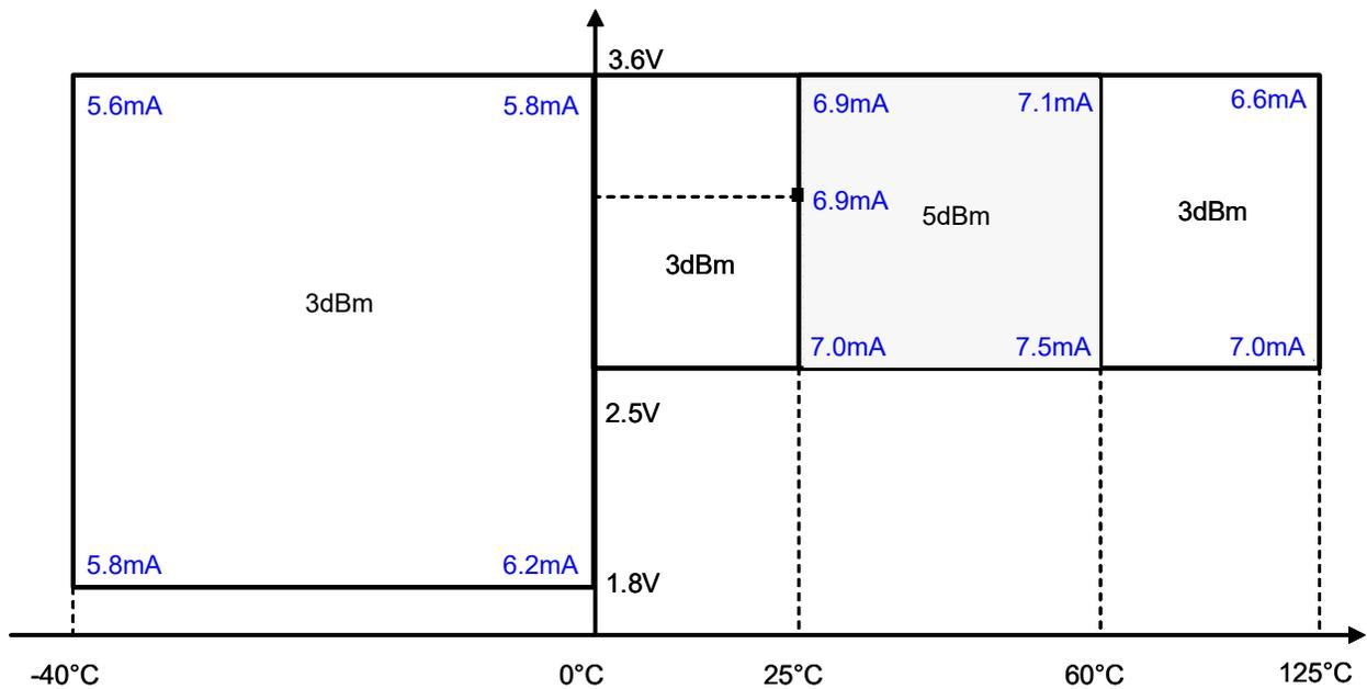
Figure 124. Dynamic Power Adjustment - 434 MHz
