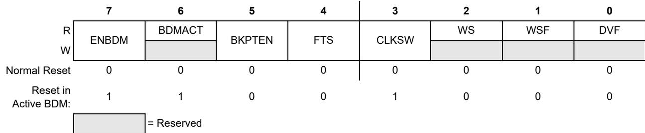
Figure 118. BDC Status and Control Register (BDCSCR)
