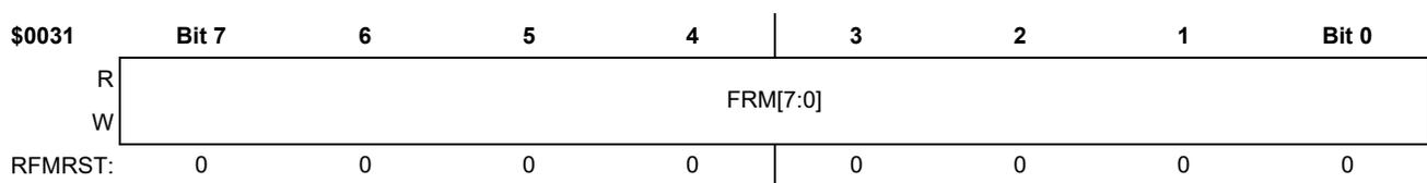
Figure 99. RFM Control Register 1 (RFCR1)
