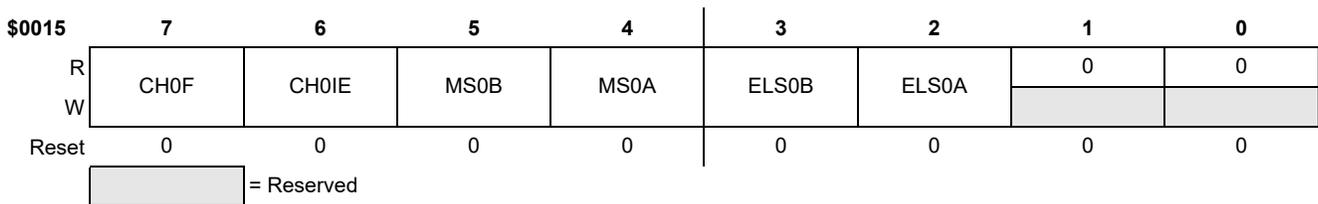
Figure 48. Timer Channel 0 Status and Control Register (TPM1C0SC)
