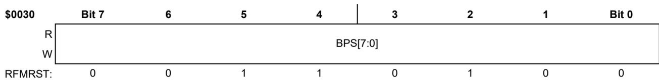
Figure 98. RFM Control Register 0 (RFCR0)
