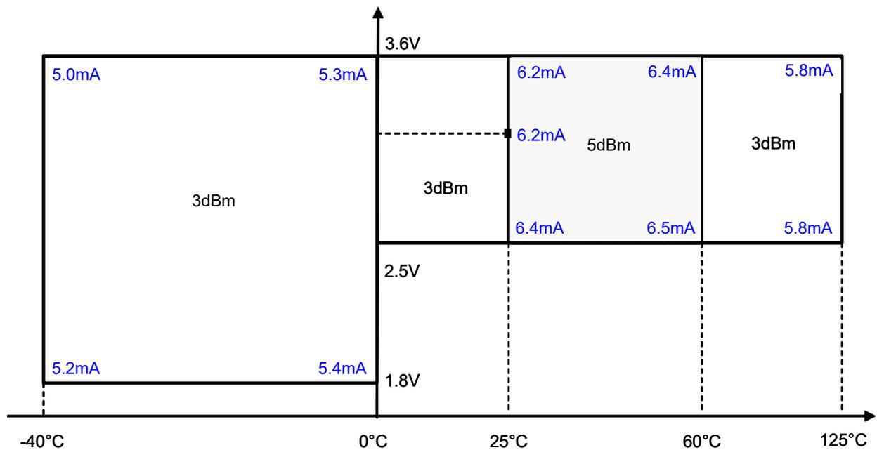
Figure 123. Dynamic Power Adjustment - 315 MHz
