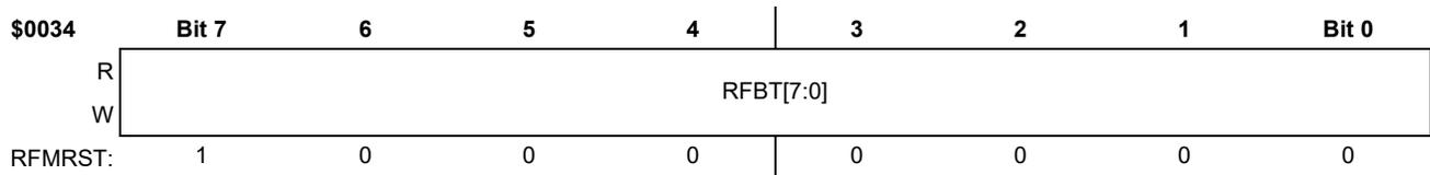
**Figure 103. RFCR4 Register - Base Time Variable**
