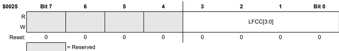
Figure 88. LFR Control Register A (LFCTRLA, LPAGE = 1)
