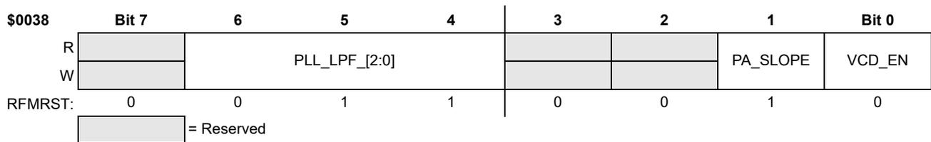
**Figure 109. RFM EPR Registers (EPR, RPAGE = 1, VCD\_EN = 0)**
