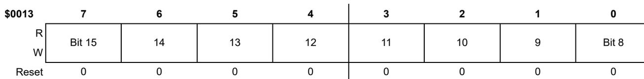
**Figure 46. Timer Counter Modulo Register High (TPM1MODH)**
