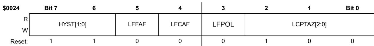
Figure 87. LFR Control Register B (LFCTRLB, LPAGE = 1)
