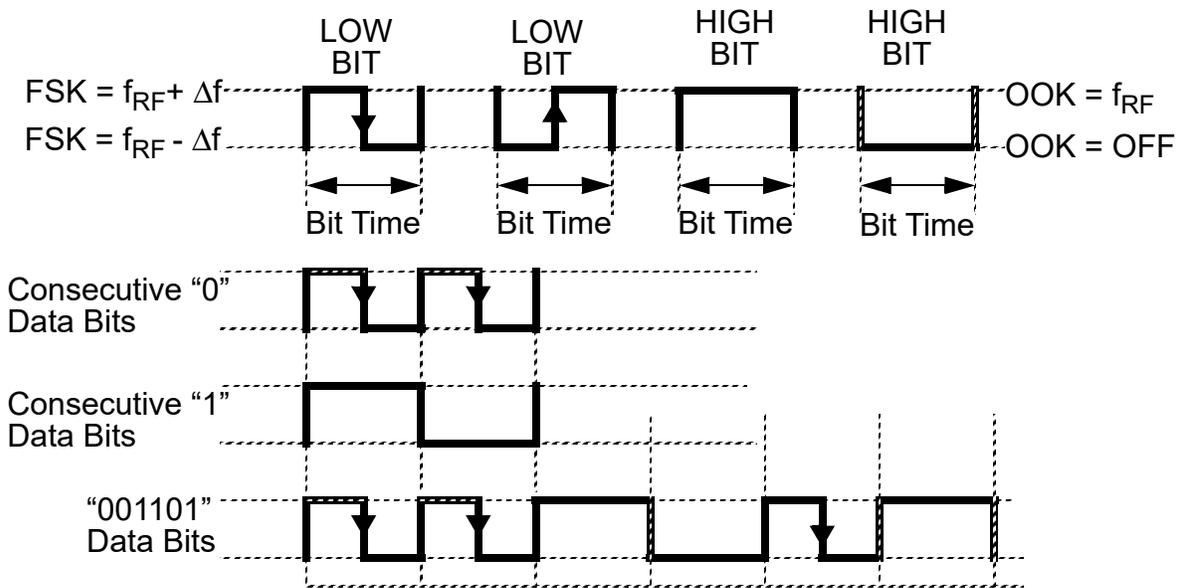
Figure 96. Bi-Phase Data Bit Encoding (POL = 0)
