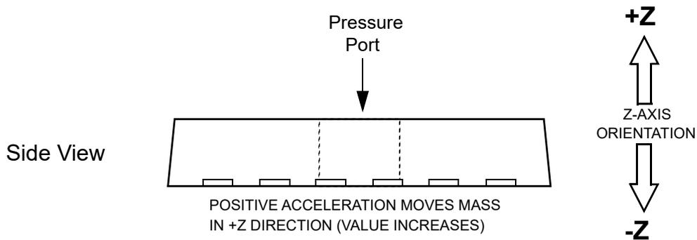
**Figure 4. FXTH871x6 QFN Optional Z-axis Accelerometer Orientation**
