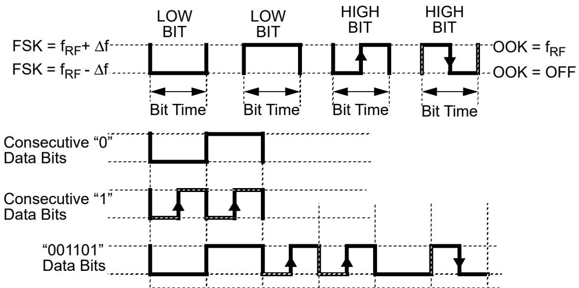
Figure 97. Bi-Phase Data Bit Encoding (POL = 1)
