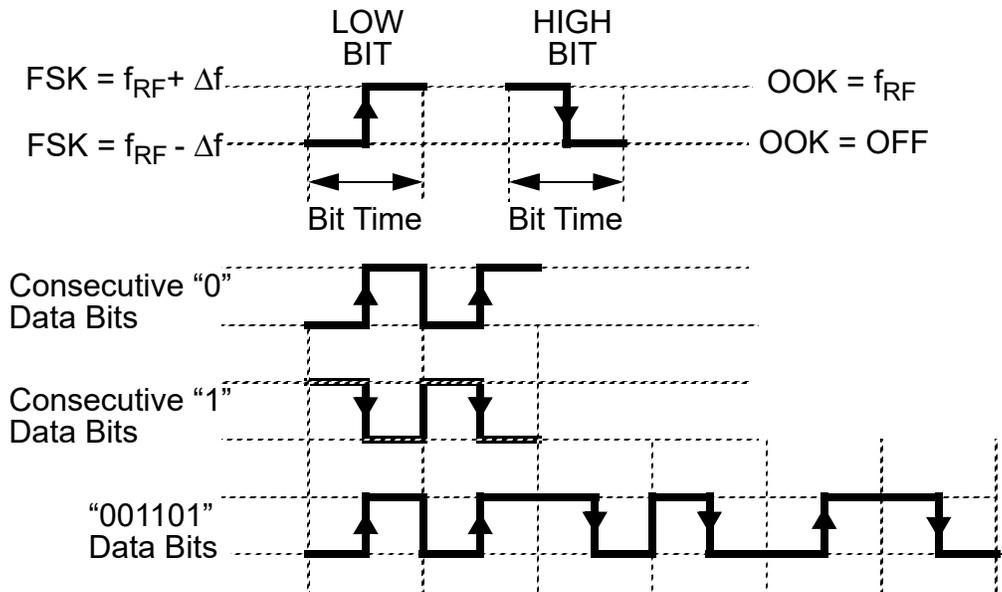
Figure 94. Manchester Data Bit Encoding (POL = 0)
