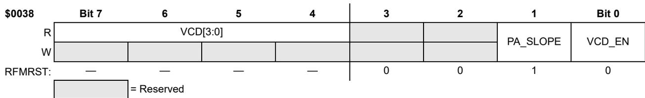
**Figure 110. RFM EPR Registers (EPR, RPAGE = 1, VCD\_EN = 1)**
