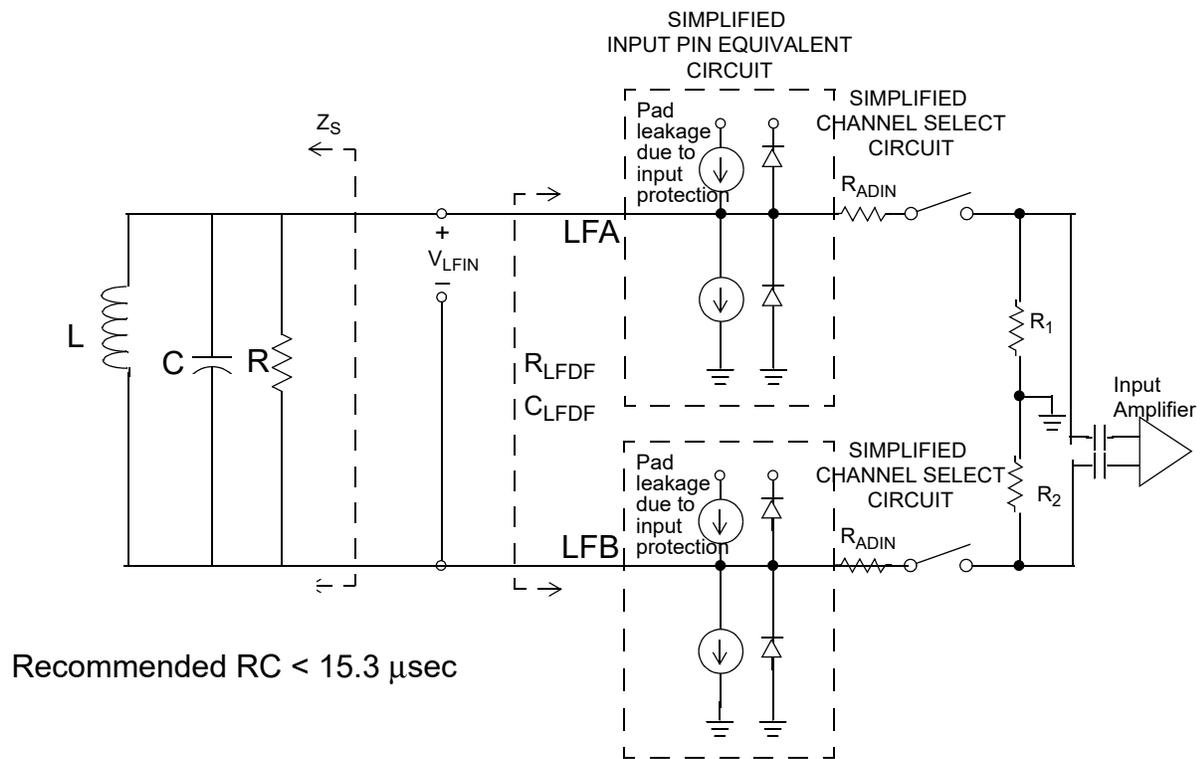
Figure 122. LFR Detector Input Equivalent Circuit
