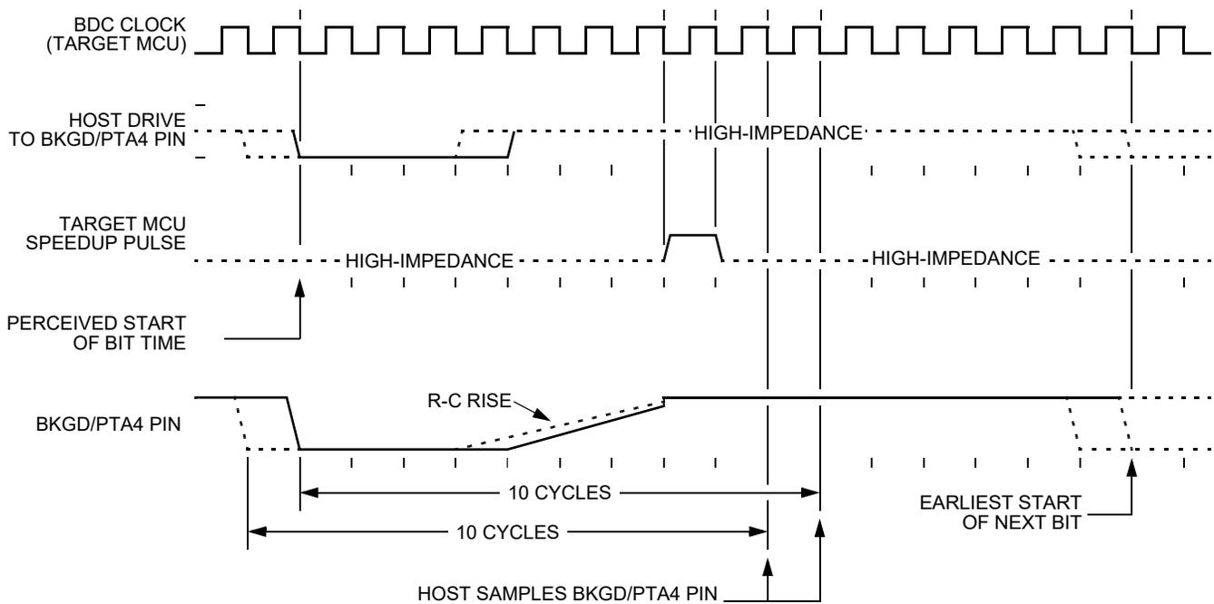
**Figure 116. BDC Target-to-Host Serial Bit Timing (Logic 1)**
