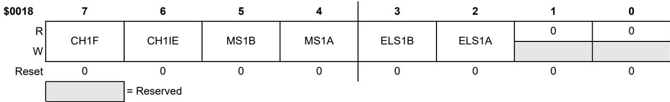
Figure 51. Timer Channel 1 Status and Control Register (TPM1C1SC)
