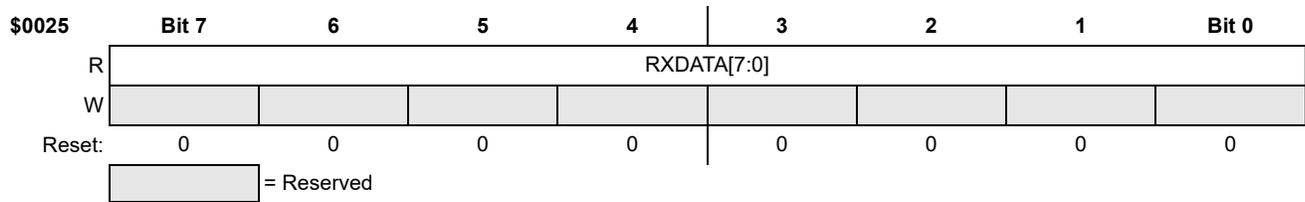
Figure 81. LFR Data Register (LFDATA) when LPAGE = 0
