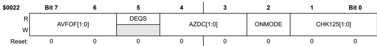
Figure 85. LFR Control Register D (LFCTRLD, LPAGE = 1)
