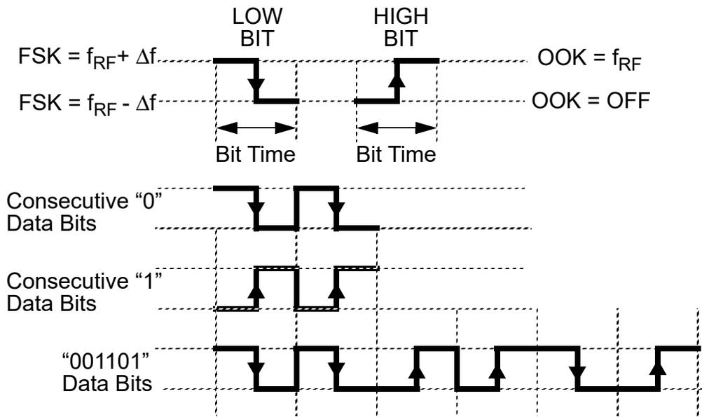
Figure 95. Manchester Data Bit Encoding (POL = 1)
