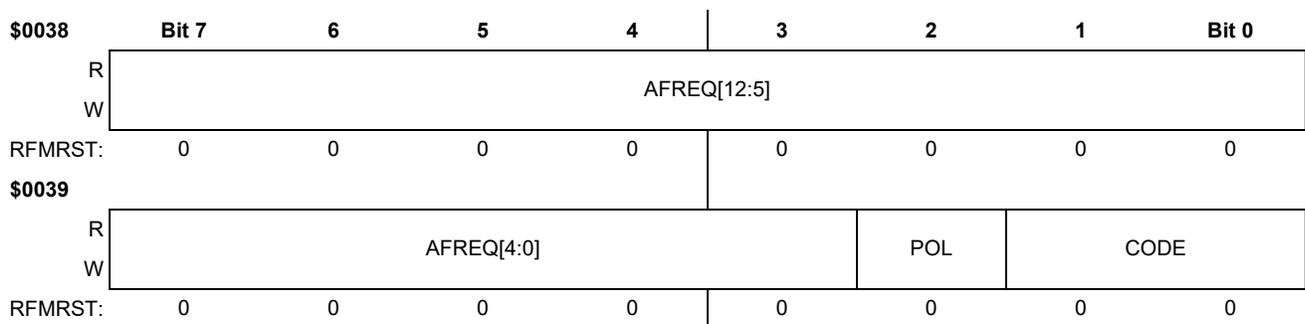
**Figure 107. PLL Control Registers A (PLLCR[1:0], RPAGE = 0)**
