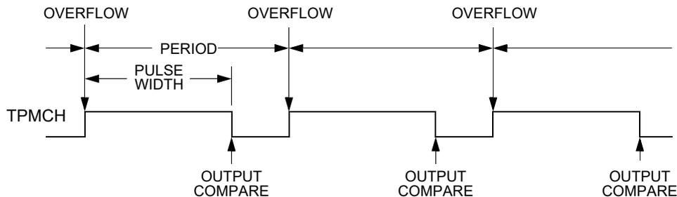
Figure 54. PWM Period and Pulse Width (ELSnA = 0)
