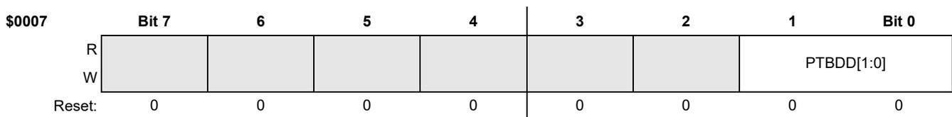
**Figure 35. Data Direction for Port B Register (PTBDD)**
