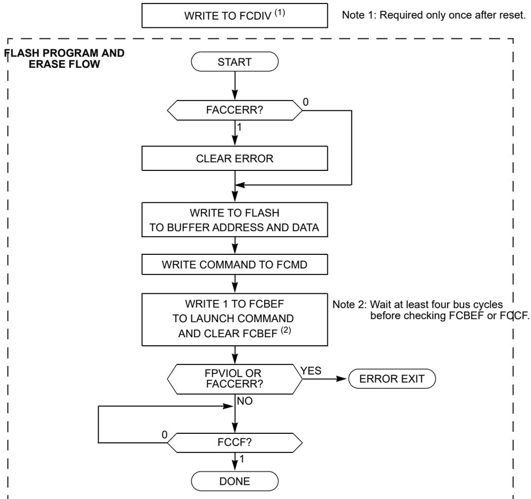
Figure 9. FLASH Program and Erase Flowchart
