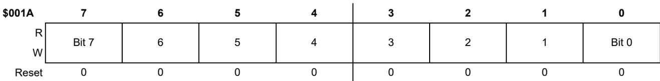
**Figure 53. Timer Channel 1 Value Register Low (TPM1C1VL)**
