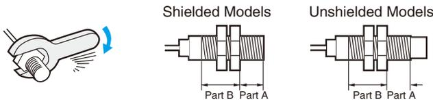
Note: 1. The allowable tightening strength depends on the distance from the edge of the head, as shown in the following table. (A is the distance from the edge of the head. B includes the nut on the head side. If the edge of the nut is in part A, the tightening torque for part A applies instead.)
