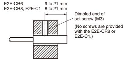
When using a set screw, tighten it to a torque of 0.2 N·m max. (E2E-C1: 0.4 N·m max.)
