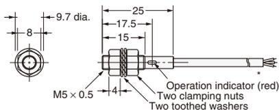
\*2.9-dia. vinyl-insulated round cable with 3 conductors (Conductor cross section: 0.14 mm<sup>2</sup>, Insulator diameter: 0.9 mm), Standard length: 2 m
