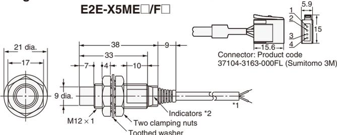
\*1. 4-dia. vinyl-insulated round cable with 2 conductors (Conductor cross section: 0.3 mm<sup>2</sup>, Insulator diameter: 1.3 mm), Standard length: 2 m
