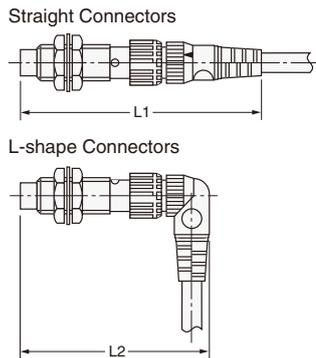
**Dimensions with the XS2F Connected (Unit: mm)**
