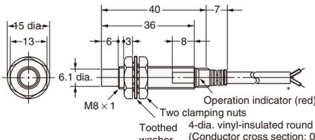
4-dia. vinyl-insulated round cable with 2 conductors (Conductor cross section: 0.3 mm<sup>2</sup>, Insulator diameter: 1.3 mm), Standard length: 2 m
