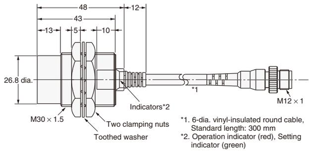
**Dimensions for Proximity Sensors with Sensor I/O Connectors**
