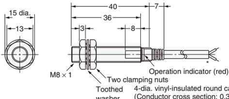
4-dia. vinyl-insulated round cable with 2 conductors (Conductor cross section: 0.3 mm<sup>2</sup>, Insulator diameter: 1.3 mm), Standard length: 2 m
