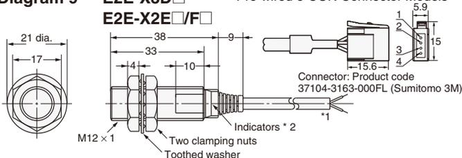
\*1. 4-dia. vinyl-insulated round cable with 2 conductors (Conductor cross section: 0.3 mm<sup>2</sup>, Insulator diameter: 1.3 mm), Standard length: 2 m
