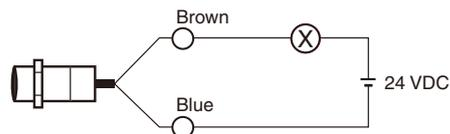
Note: DC 2-Wire Sensors have a residual voltage of 3 V. Check the operating voltage of the relay before use.
