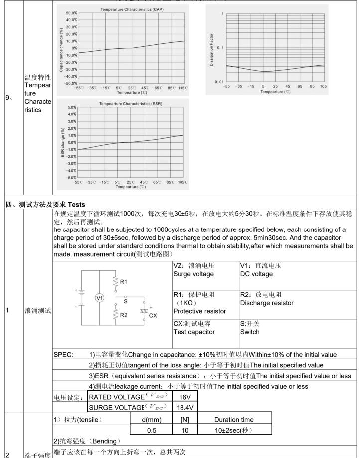
The terminal shall be subjected to 1 bend in each direction to give a total 2 bends.
