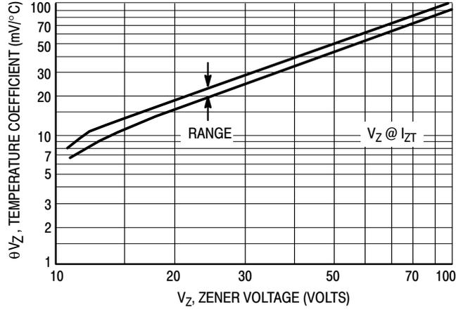
**Figure 2. Temperature Coefficients**
