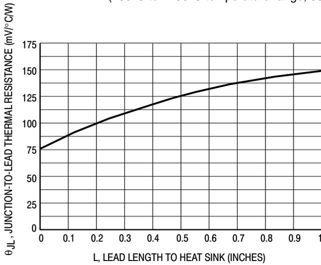
**Figure 3. Typical Thermal Resistance versus Lead Length**
