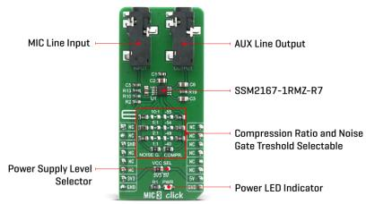
The Click board™ provides four different preset values of the compression ratio. Changing the scaling of the control signal fed to the VCA causes a change in the circuit compression ratio.Lowering RCOMP gives smaller compression ratios as indicated in Table. Automatic Gain Control (AGC) performance is achieved with compression ratios between 2:1 and 10:1, and is dependent on the application. Shorting RCOMP disables the AGC function, setting the compression equal to 1:1.
