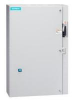
Non-reversing motor starter, Size 4, Three phase full voltage, Solid-state overload relay, OLRelay amp range 50-200A, 110V 50HZ / 120V 60HZ coil, Combination type, 200A non-fusible disconnect, Enclosure NEMA type 1, Indoor general purpose use, Standard width enclosure
