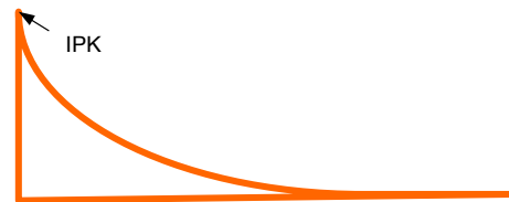
Figure 26. Input Charge Inrush Current
