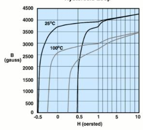
Measured on a 13/8/6mm toroid at 10 kHz.
