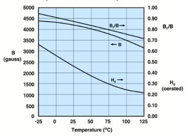
Measured on a 13/8/6mm toroid at 10 kHz. B is measured at H=10 oersted.
