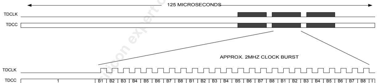
The Transmit Section Data Link Clock and Data Insertion diagram (Figure 48) shows the relationship between the TDCC serial data input, and its associated TDCLK. In this mode, TDCLK is a 216 kHz, 50% duty cycle clock that is gapped to produce a 192 kHz nominal rate. TDCC is sampled on the rising edge of TDCLK. The D1-D3 bytes shifted in to the S/UNI-1x155 in the frame shown are inserted in the corresponding transport overhead channels in the next frame.
