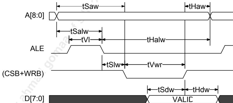
**Notes on Microprocessor Interface Write Timing:**
