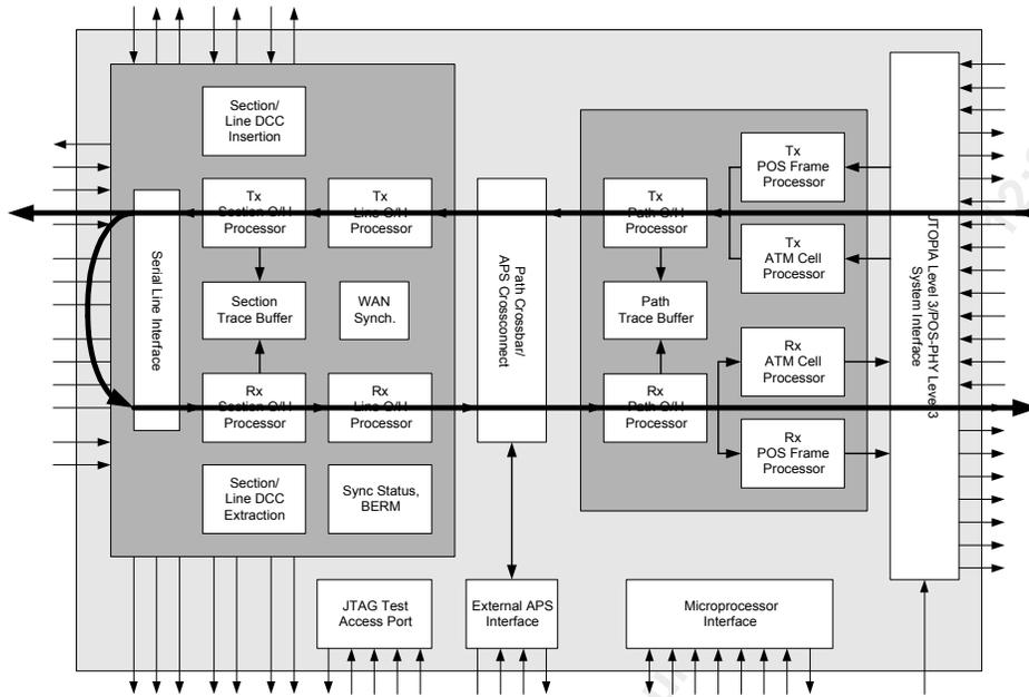
**Figure 24 Parallel Diagnostic Loopback Mode**
