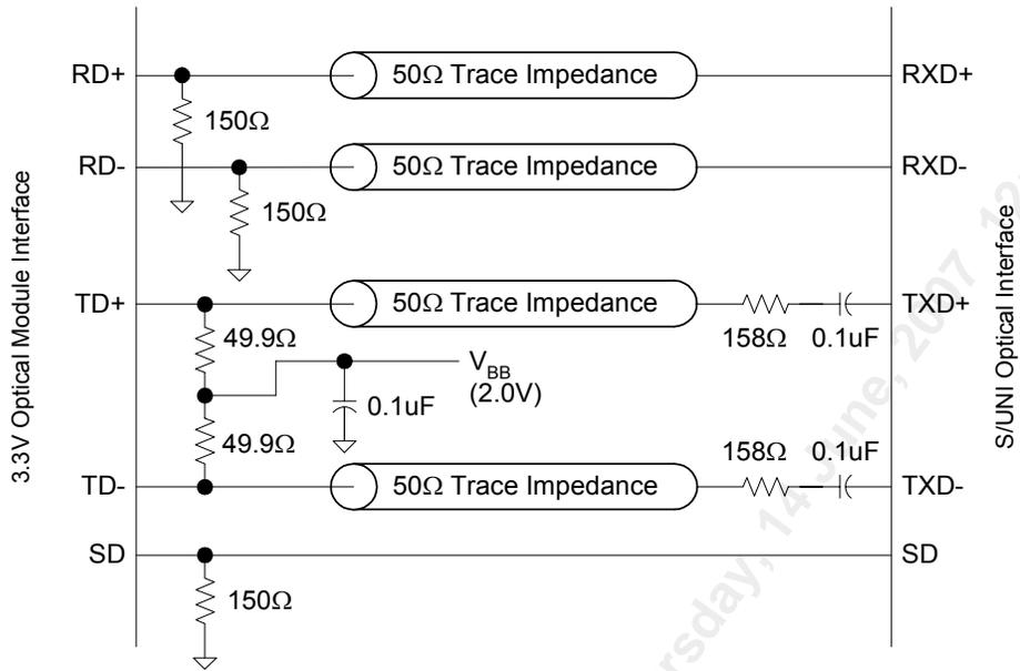
**Figure 34 Interfacing S/UNI-1x155 Line PECL Pins to 5.0V Devices**
