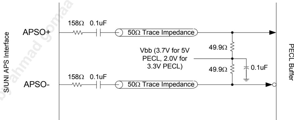
**Figure 37 APS Input Interface from PECL buffer**
