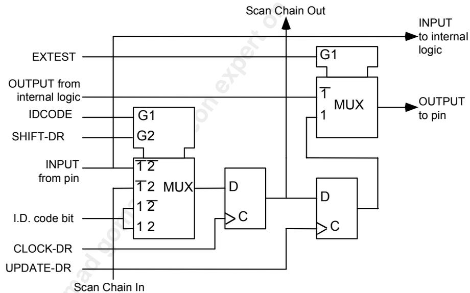
**Figure 14 Layout of Output Enable and Bidirectional Cells**
