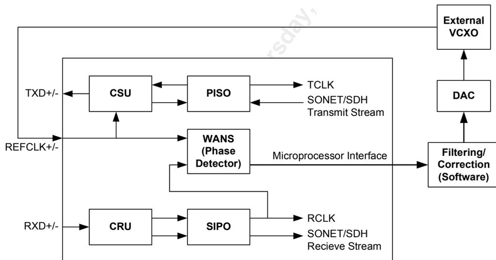
The software running on the external processor is responsible for performing: digital loop filtering, temperature compensation, VCXO linearity compensation; determining the validity of the timing reference; and performing reference switchover. The VCXO creates the 19.44 MHz Stratum 3 reference clock which the CSU will synthesize to the desired 155.52 MHz transmit clock.
