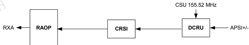
Because of the architecture of the receive APS interface, the reference clocks REFCLK for both S/UNI-1x155 must be frequency locked. While the DCRU can track jitter on the serial interface, the DCRU cannot process serial interfaces with a frequency offset from the 155.52 MHz clock synthesized by the CSU block.
