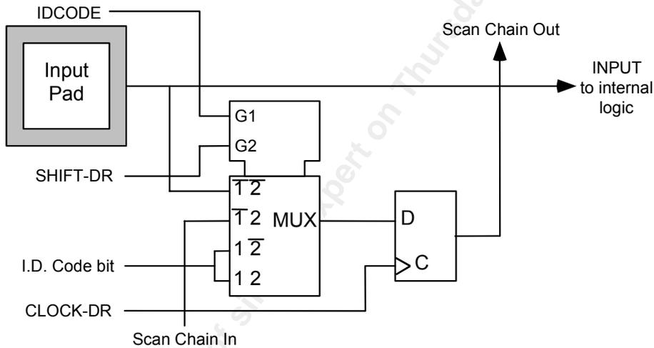
**Figure 12 Output Cell (OUT\_CELL)**
