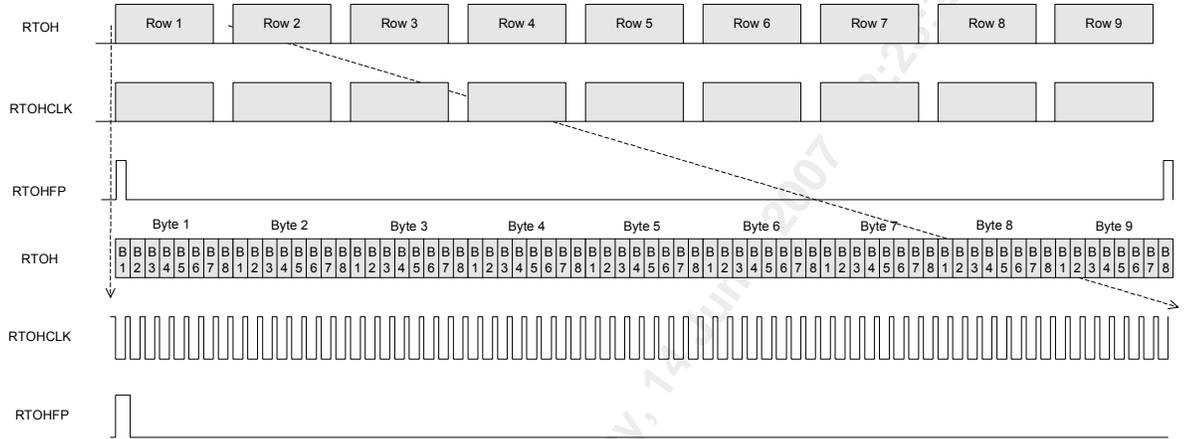
The transport overhead extraction timing diagram above illustrates the transport overhead extraction interface for STS-3c (STM-1). The transport overhead extraction clock, RTOHCLK is nominally a 5.184 MHz clock and is derived from the receive line clock, RCLK. The entire transport overhead (the complete 9 row by 9 column structure) is extracted for the STS-3c (STM-1) stream and is serialized on RTOH over a frame period (125 µs).
