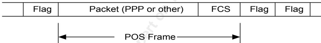
In the event of a FIFO overflow caused by the FIFO being full while a packet is being received, the packet is marked with an error so it can be discarded by the system. Subsequent bytes associated with this now aborted frame are discarded. Reception of POS data resumes when a Start of Packet is encountered and the FIFO level is below the programmable Reception Initialization Level (RIL[7:0]).
