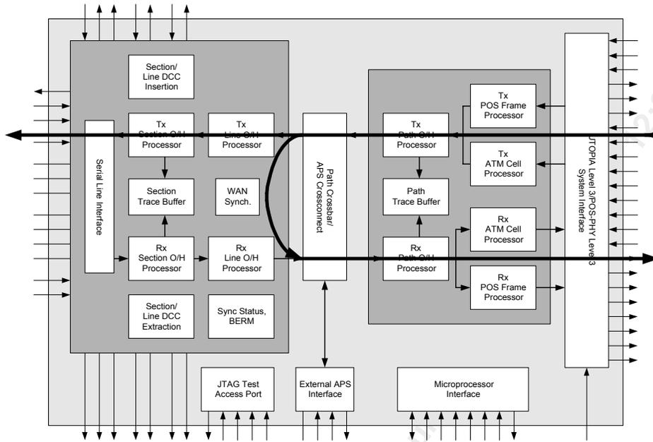
**Figure 26 Data Diagnostic Loopback Mode**
