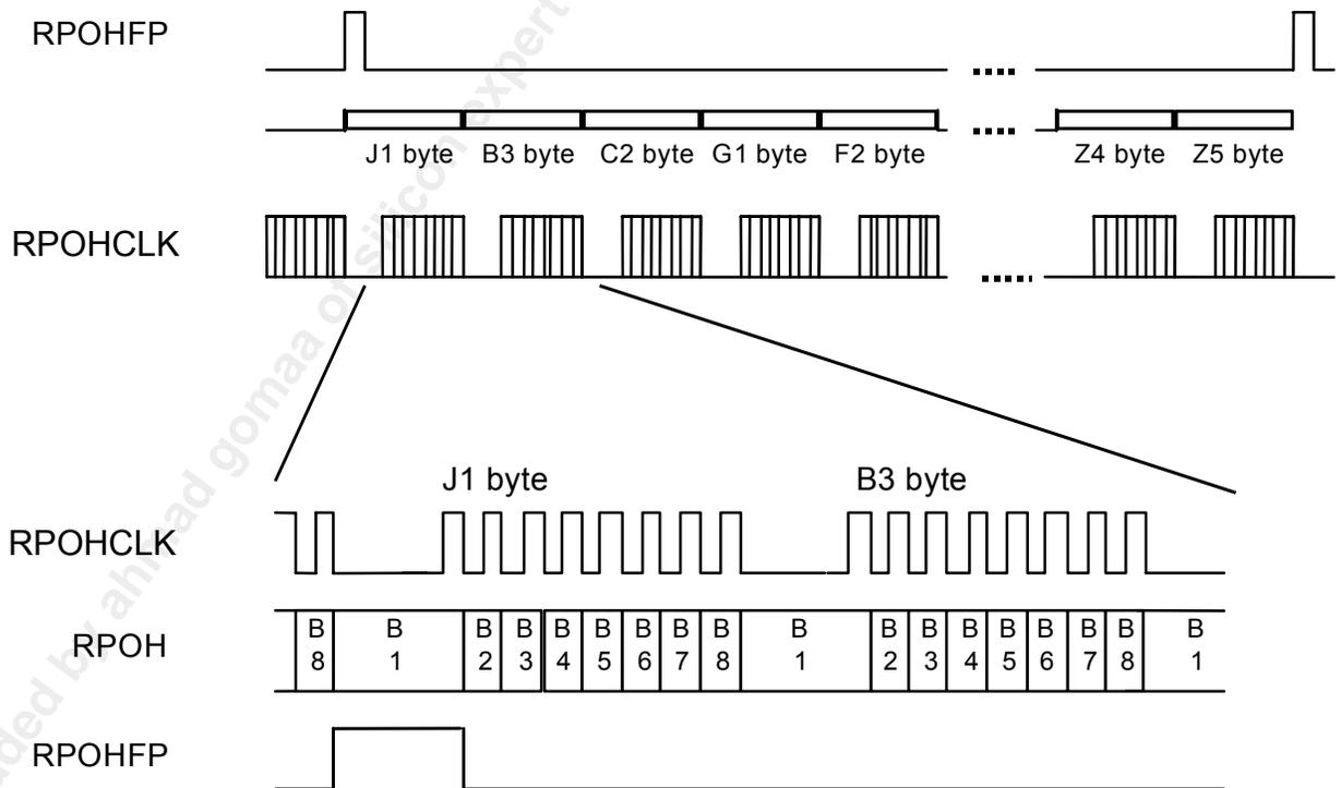
The figure above shows the receive path overhead extraction to a low speed serial stream. RPOHCLK are nominally 576 KHz clocks. The entire path overhead (J1, B3, C2, G1, F2, H4, Z3, Z4, Z5 bytes) is extracted, serialized and placed on RPOH over a frame period. For each byte, the most significant bit is transmitted first. RPOHFP mark the most significant bit of the J1 byte.
