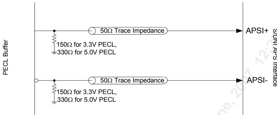
**Figure 38 APS Interface between two PM5384 devices**
