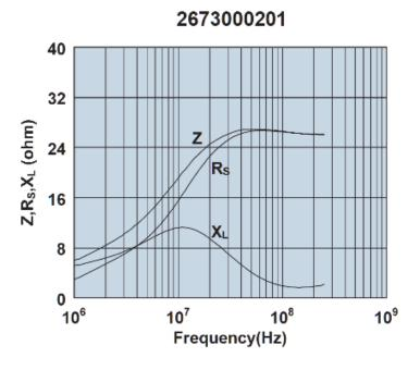
Impedance, reactance, and resistance vs. frequency.
