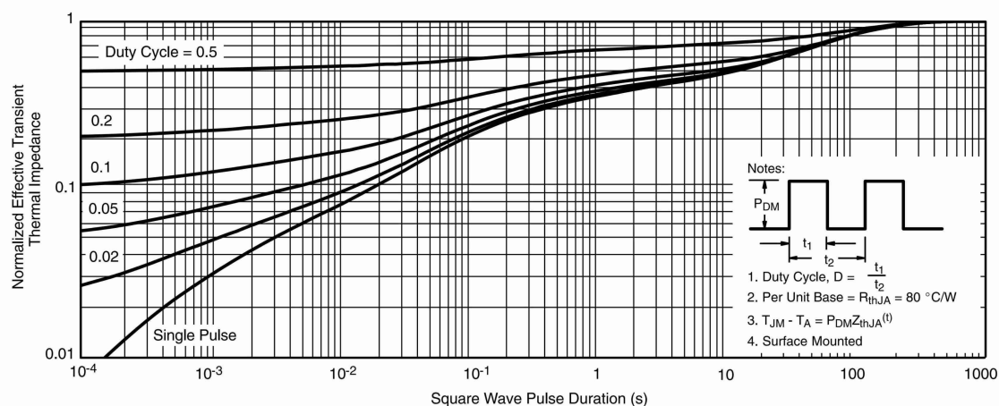
Normalized Thermal Transient Impedance, Junction-to-Ambient
