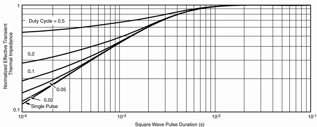
Normalized Thermal Transient Impedance, Junction-to-Case
