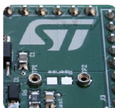
Figure 4. Mounting through-hole sense resistor
