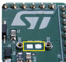
Figure 5. Pads for soldering SMD resistor
