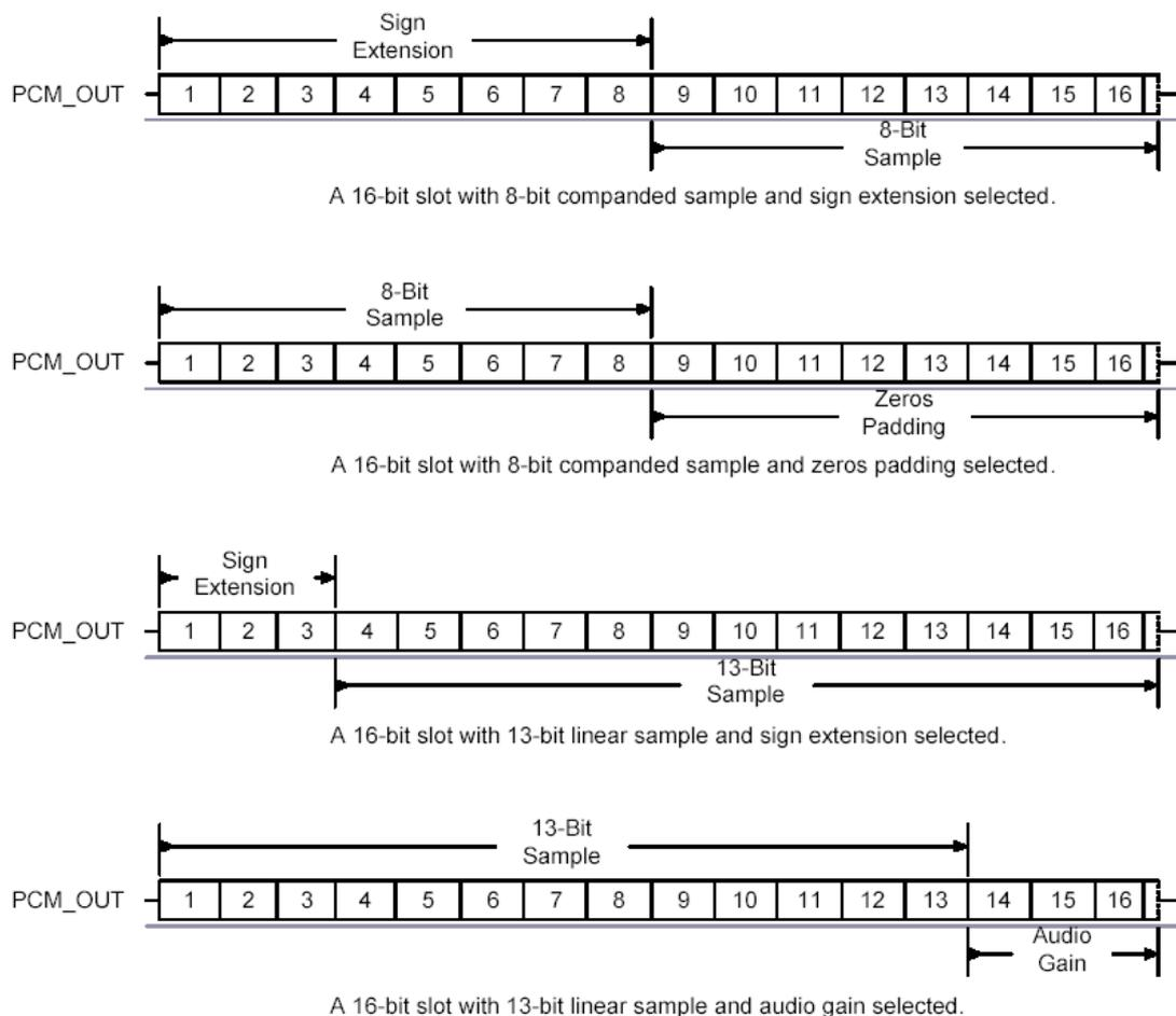
**Figure 19: 16-bit Slot Length and Sample Formats**
