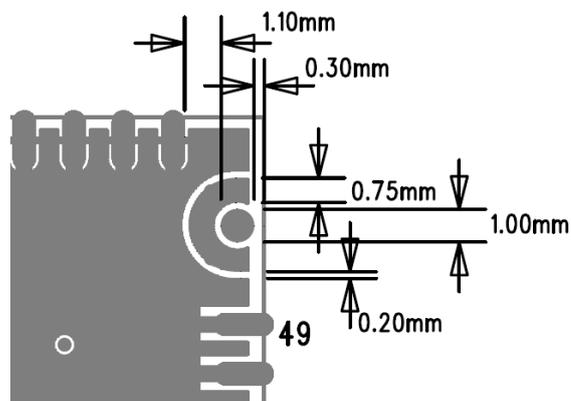
Figure 3: Dimensions for the RF pin (top view)
