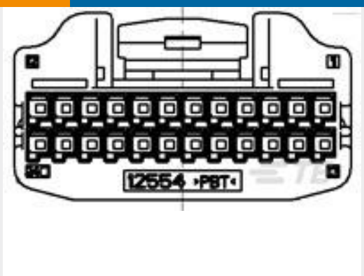
TE Part #1717112-2 0.64 III 24POS PLUG ASSY
