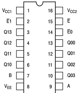
Pin assignment is for Dual-in-Line Package.
