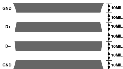
Figure 19. Arrangement of Signal Tracks
