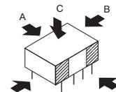
Please chuck the portion. Avoid chucking the center of the relay. In addition, excessive chucking pressure to the pinpoint of the relay should be also avoided.
