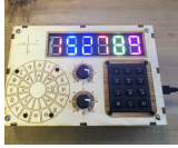
Mystery Box: NeoMatrix Mk I Interface of Infinite Possibilities: Matrix keypad and NeoSegment display
