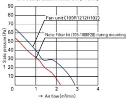
Applied voltage: DC12V Note: Measuring with the fan suction side-fitted filter kit
