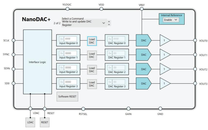
Figure 4. Chip Block Diagram View of the AD5686R or the AD5696R
