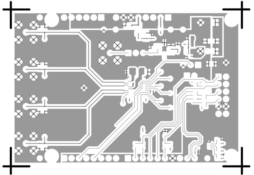
Figure 11. NanoDAC+ Evaluation Board—Top Side Routing
