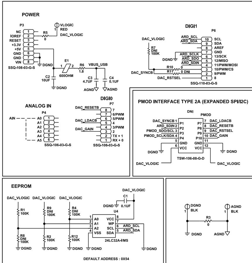
Figure 9. NanoDAC+ Evaluation Board Schematic Diagram—SDP Connector, PMOD, and EEPROM
