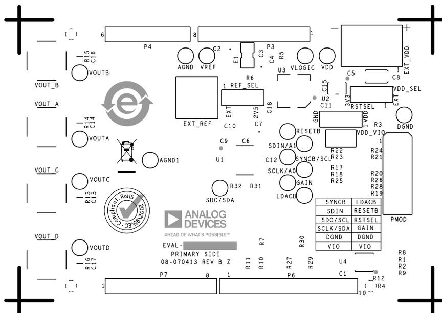
Figure 10. NanoDAC+ Evaluation Board—Component Placement
