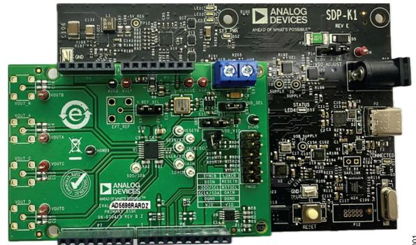
Figure 1. Evaluation Board Connected to the SDP-K1 Controller Board (EVAL-AD5686RARDZ or EVAL-AD5696RARDZ)
