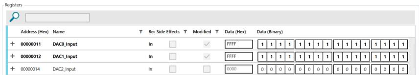
**Figure 7. Memory Map of the AD5686R or the AD5696R with Pending Changes in the DAC0\_Input Register**
