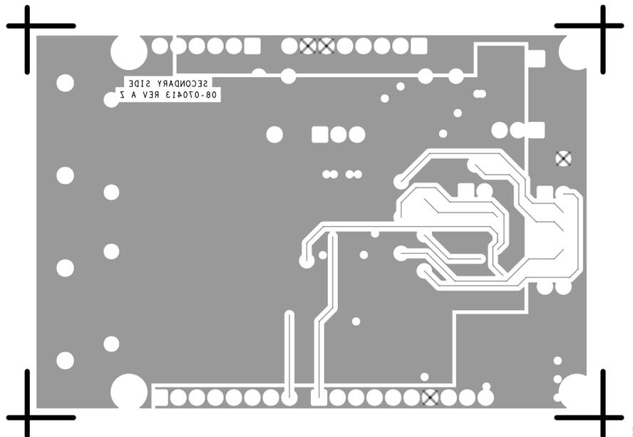
Figure 12. NanoDAC+ Evaluation Board—Bottom Side Routing
