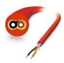
Polymer fiber cable, duplex 980  $\mu\text{m}/1000~\mu\text{m}$ , medium-weight version for installation in stationary systems and machines, by the meter without male connector
