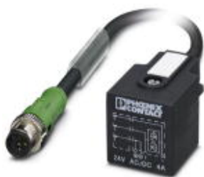
Sensor/actuator cable, 3-position, PUR/PVC, black RAL 9005, Plug straight M12 SPEEDCON, A-coded, on Valve connector A, with 1 LED, connected with Z diode, cable length: 3 m
