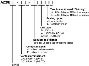
00: Flange mount, QC terminals on top 50: PCB mount, solder terminals
